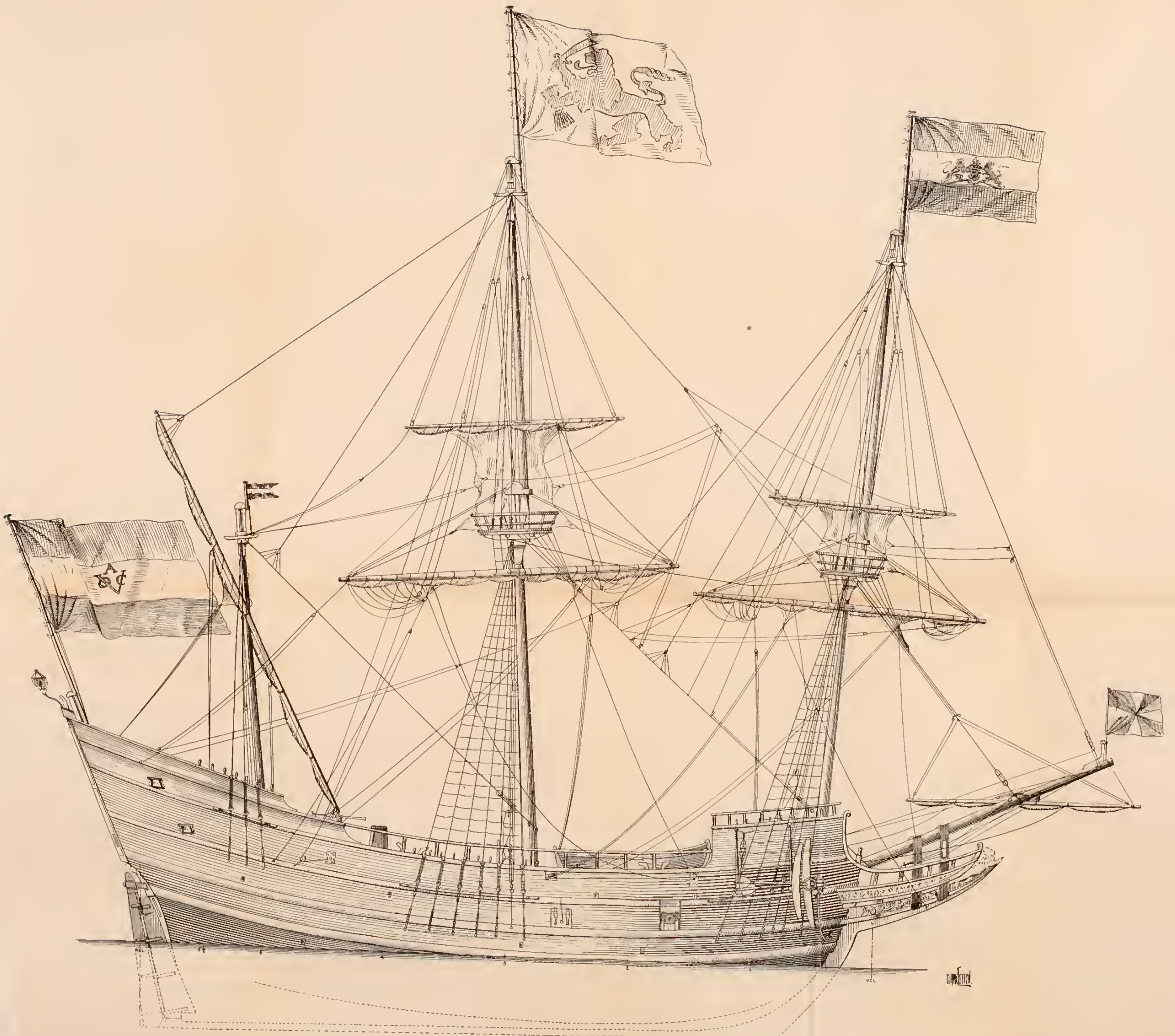
THE HALF MOON. PLAN OF RIGGING. SCALE, 1:80.
